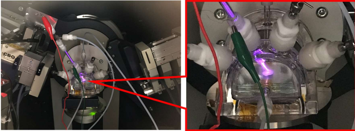
Fig. 2. In situ XRD during plasma irradiation
