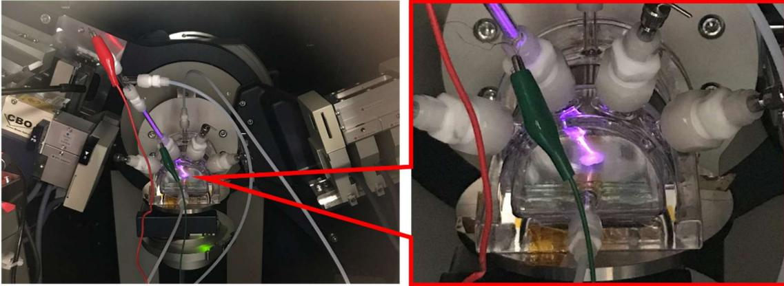
Fig. 2. *In situ* XRD during plasma irradiation
