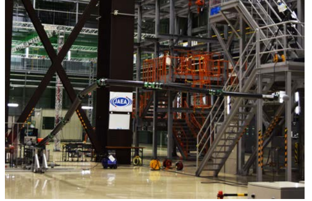
Fig. 1. Super Dragon: a 10-m-long coupled tendon-driven articulated manipulator [1].
