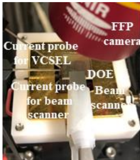
Fig. 3-20 Setup to measure the beam scanner integrated to a conventional VCSEL
