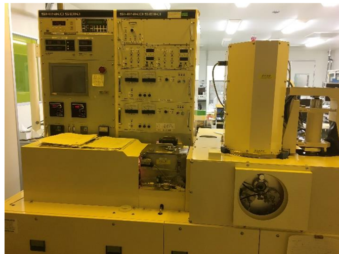
Fig. 2-8 Material sputtering machine
