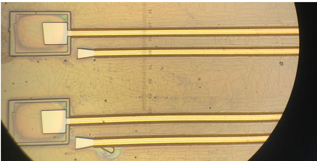
Fig. 2-13 The photo of fabricated solitary beam scanner
