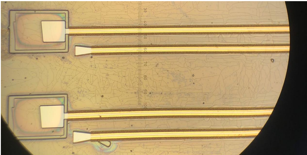
Fig. 2-13 The photo of fabricated solitary beam scanner
