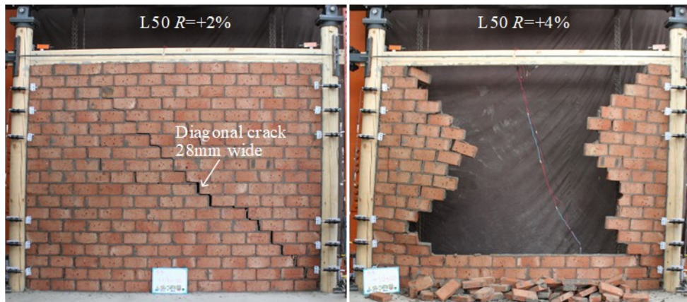
Figure 3-17. Shear cracking and collapse of masonry infill in specimen L50.
