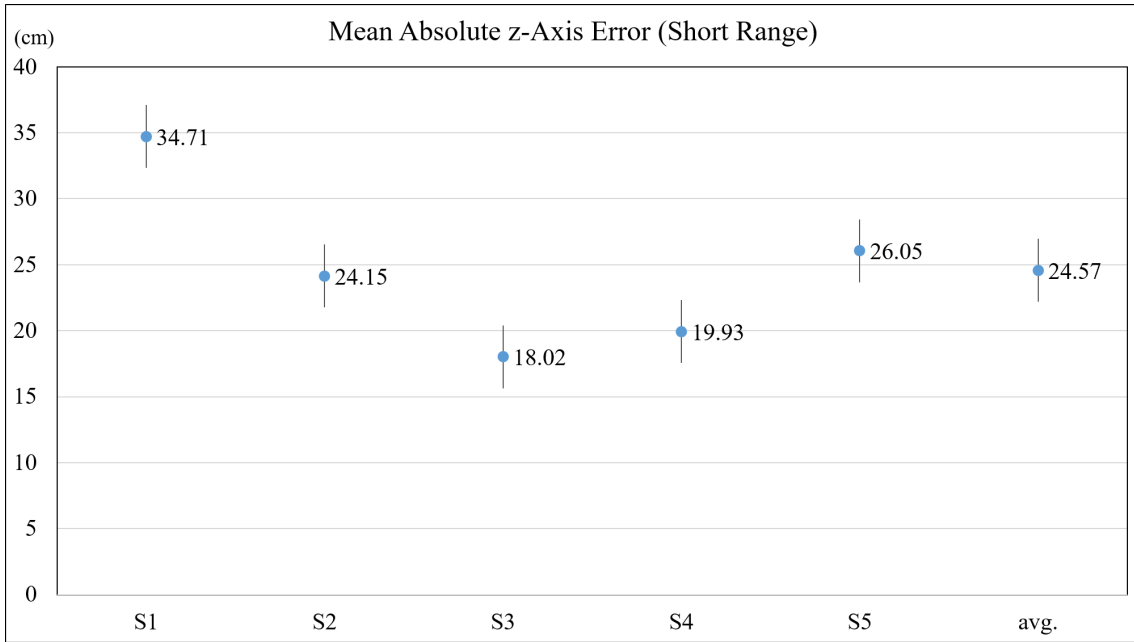
Figure 5.8: Mean absolute error of depth estimation for each subject in a short-range space.
