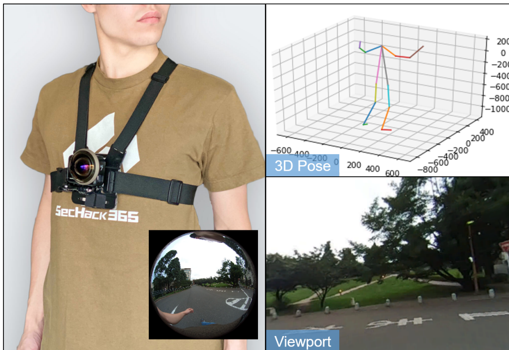
Figure 3.1: Our multimodal human motion capture system is based on a single ultra-wide fisheye camera that is worn on the user’s chest. The wearable hardware configuration of MonoEye enables activity capture in everyday life.
