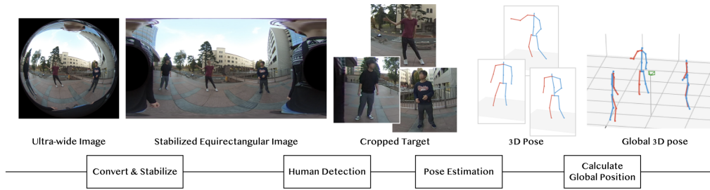
Figure 3.7: Overview of the proposed pipeline. Converting into an equirectangular image, human detection, and pose estimation are applied. Then, the targets’ locations are calculated to obtain global 3D poses.
