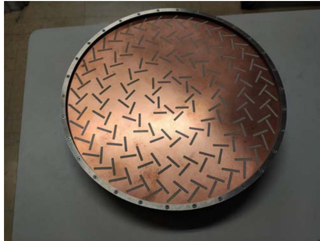
Figure 3.15: Prototype dog-bone cross-slot fed RLSA
