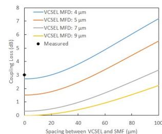
Fig. 3. Calculated/measured coupling loss from VCSEL to SMF.
