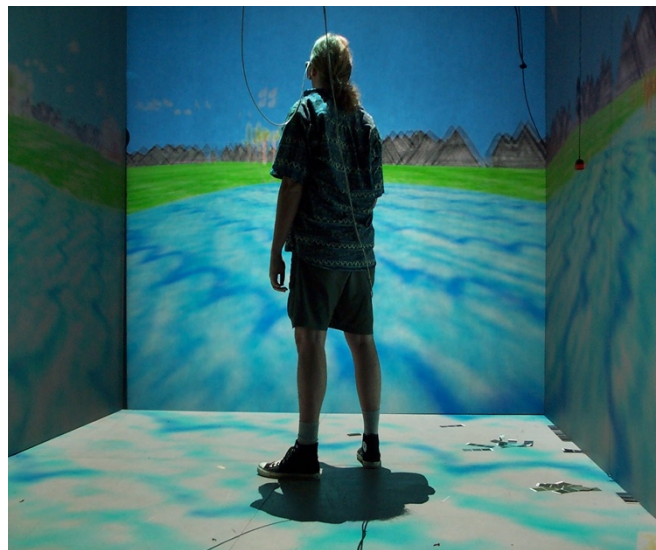
Figure 8: CAVE virtual reality environment: synchronized video projectors seamlessly project onto all walls of a room to generate a feeling of spatial immersion.
