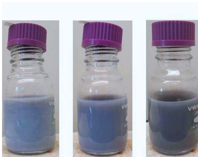
Figure 3-5. Photos of color change of the solutions during the acidic deposition of SGO composite.
