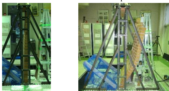
Complete slide Collapse Photo 2 Slipping and failure of the specimen
