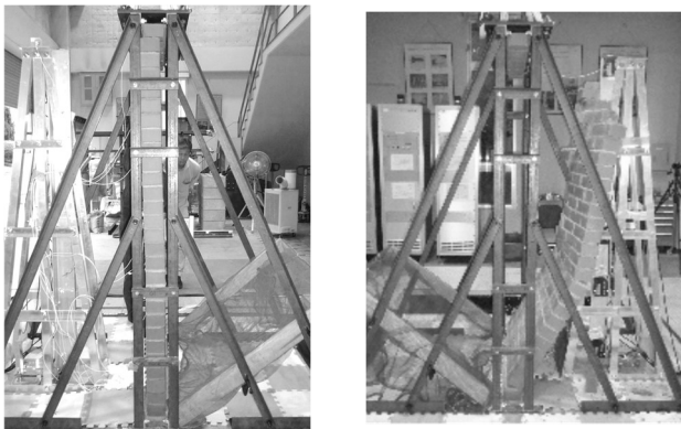
(a) Ultimate state (75% excitation) (b) Collapse (100% excitation)
