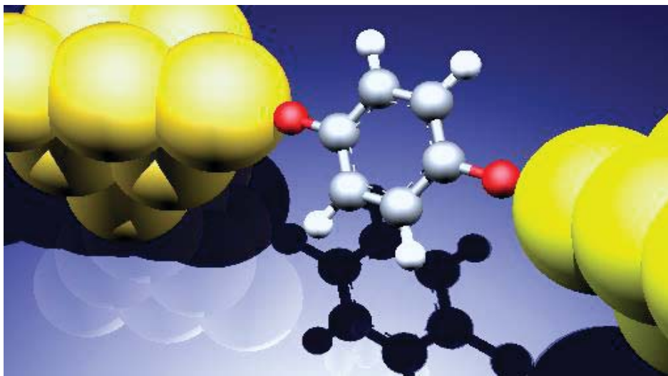
Fig.1-1 . Schematic image of single-molecule junction. Single molecule binds to two metal electrodes.
