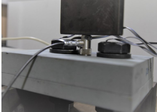
Figure 4.25 Ultrasonic measurement with constant pushing force of the probe
