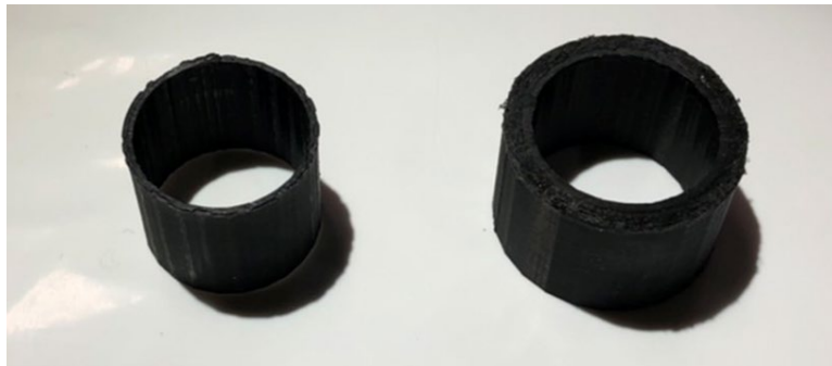
Figure 3.37 Tool for placing the bolt in the center of the bolt hole
