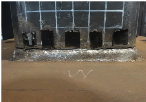
Fig. 3-3 Failure mode (flange fracture) in the experiment.
