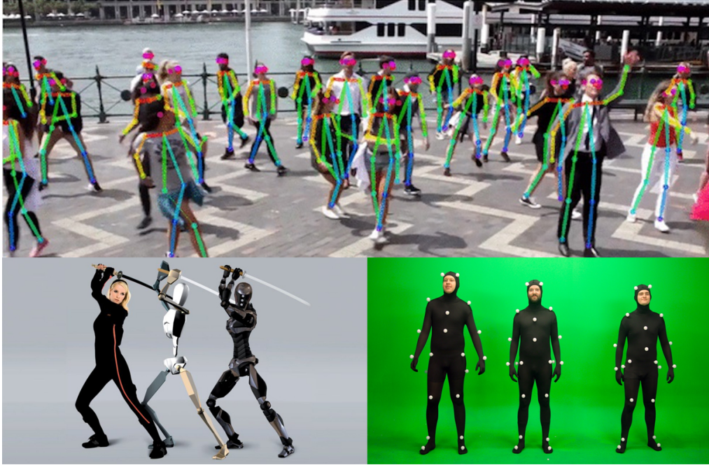
Figure 1.1: Examples of motion capture technologies: optical marker-based Optitrack [49] (upper), IMU sensor-based Xsens [52] (lower left), and depth camera based Microsoft Kinect [80].
