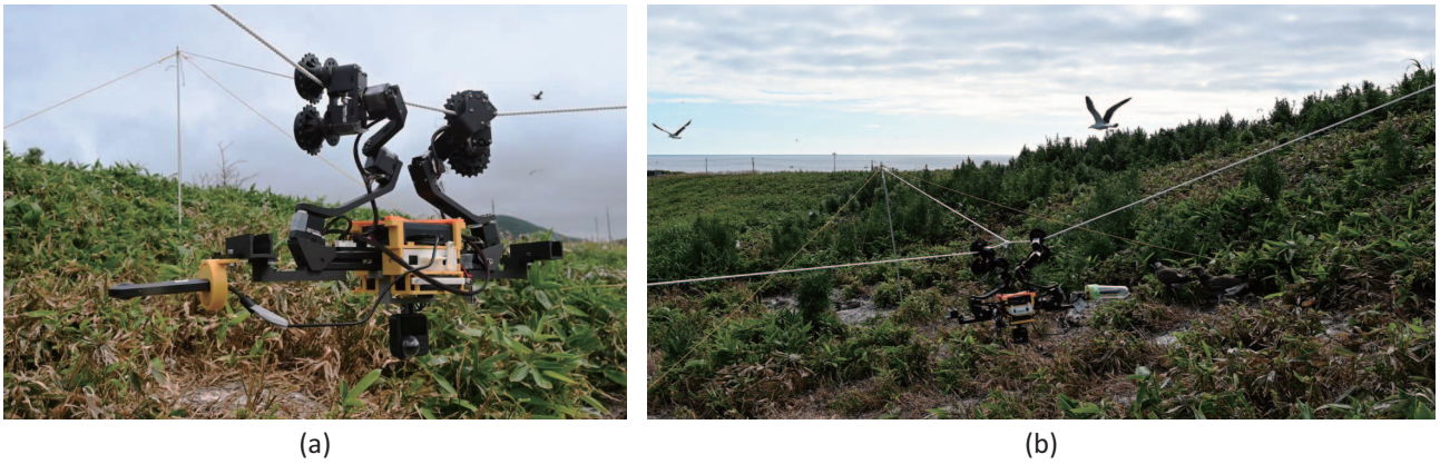
Fig. 5: TCC80DR (Tokyo Tech Cableway Crawler - No. 80 Double-arm type Refined) and its operation experiment at black-tailed gull colony on Rishiri Island (July 2022).
