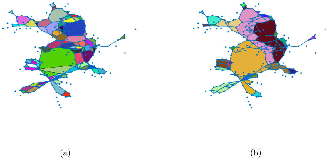
Figure 4.9: Decomposition of the IEEE 300-bus system using the (a) proposed method (b) MST method.
