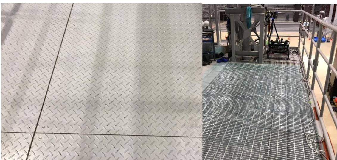
Figure 3.15 The environment setup variation in the external floor. Left: Original ground floor; Right: Floor covered with printed textures of grating lattices.
