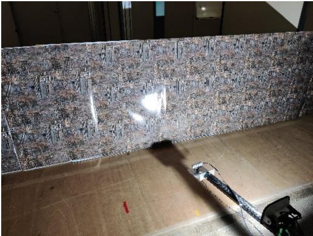
Figure 0.1 Illumination condition variation 3 with LED illumination device mounted on J3.
