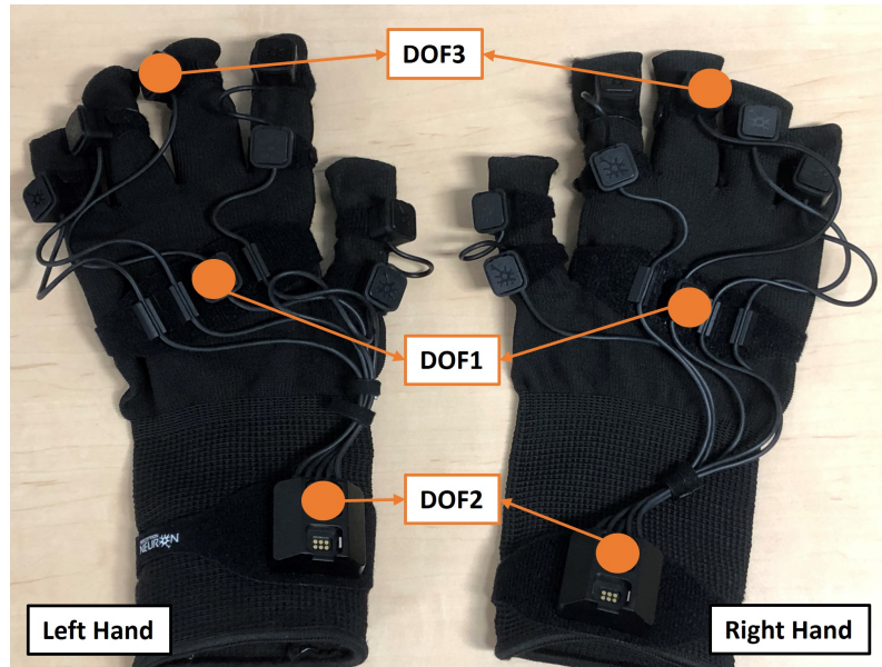
Figure 2.8: Perception Neuron Motion Capture System glove (both hands) for joint angles collection. The orange markers can obtain the joint angles from different DOFs.
