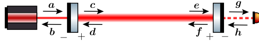
Fig. 3.4: Schematic of the Fabry-Perot cavity. The end mirror is supposed to work as a test mass.
