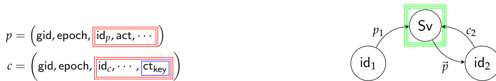
FIGURE 5.1: (Left) p and c are proposals and commits. (Right) id_1 uploads a proposal p_1 to the server Sv ; id_2 downloads all the stored proposals \vec{p} and uploads a commit c_2 for the next epoch. The single (resp. double, triple ) bordered box indicates the 1st (resp. 2nd, 3rd) layer information.
