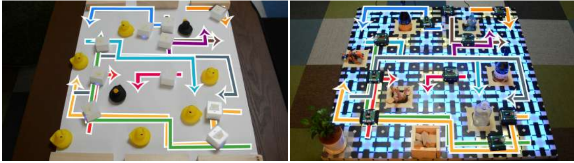
Figure 9.20: OTIMAPP execution with 10 robots in an 8 \times 8 grid. Colored arrows represent an OTIMAPP solution.
