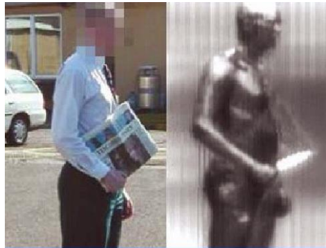
Fig. 1.3.3 Demonstration of security body scanning using THz imaging (adopted from D. Clery, Science , vol. 297, 763, 2002. [1.14]).
