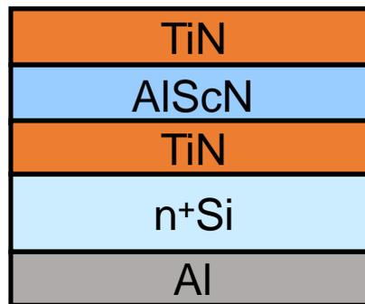
Figure 3.2 A schematic illustration of the fabricated AlScN MIM capacitor.
