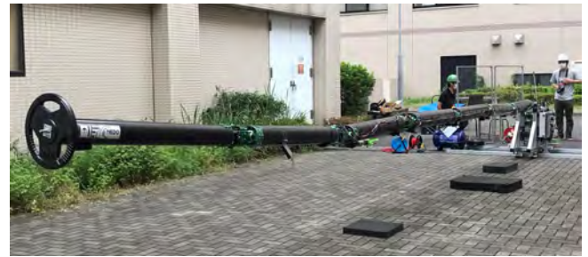
Fig.2 Power consumption testing of Super Dragon in horizontal posture with 10 kg payload.
