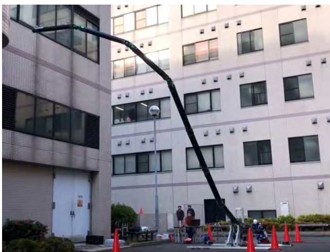
Fig.1 10-meter coupled tendon-driven super-long articulated arm for decommissioning of Fukushima Daiichi Nuclear Power Plant "Super Dragon".
