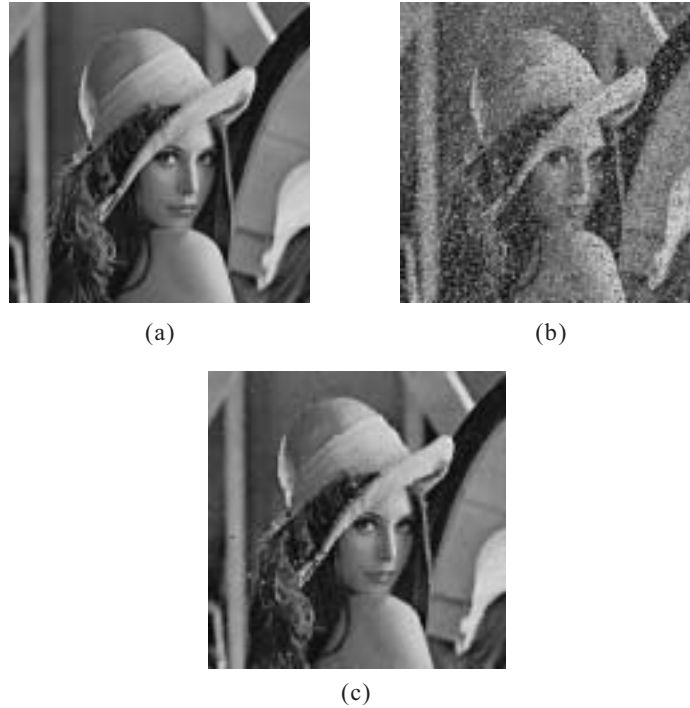
FIG. 6.5. Restoration of 256-level image by the Potts model: (a) original image, (b) degraded image, and (c) restored image. Courtesy of Kazuyuki Tanaka (1999). (Copyright 1999 by the Physical Society of Japan)
