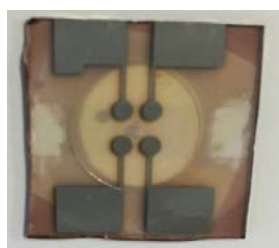
Figure 3.1. PC 71 BM structure
