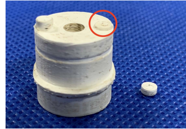
Fig.4 Break of eccentric shaft
