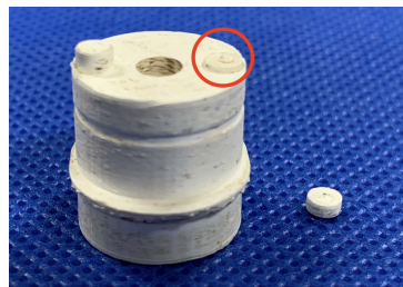
Fig.4 Break of eccentric shaft
