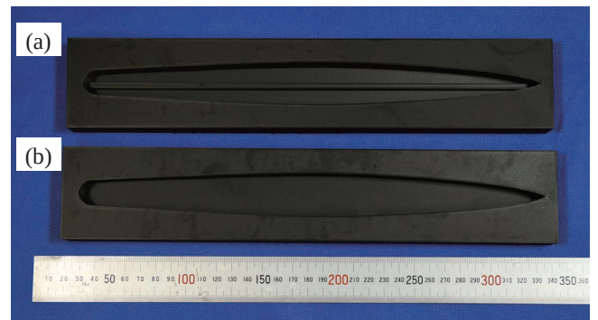
Fig.2 (a) The mold for producing grooved silicone rubber leg. (b) The mold for integrating silicone rubber and thin McKibben artificial muscle.
