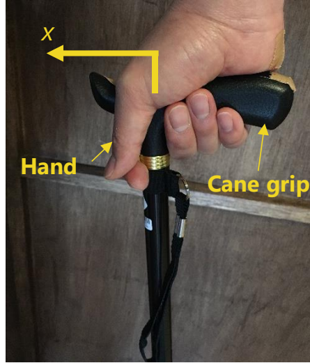
Fig. B.1: Experimental apparatus of preliminary experiment for measurement of possible slippage between a cane grip and a human hand.
