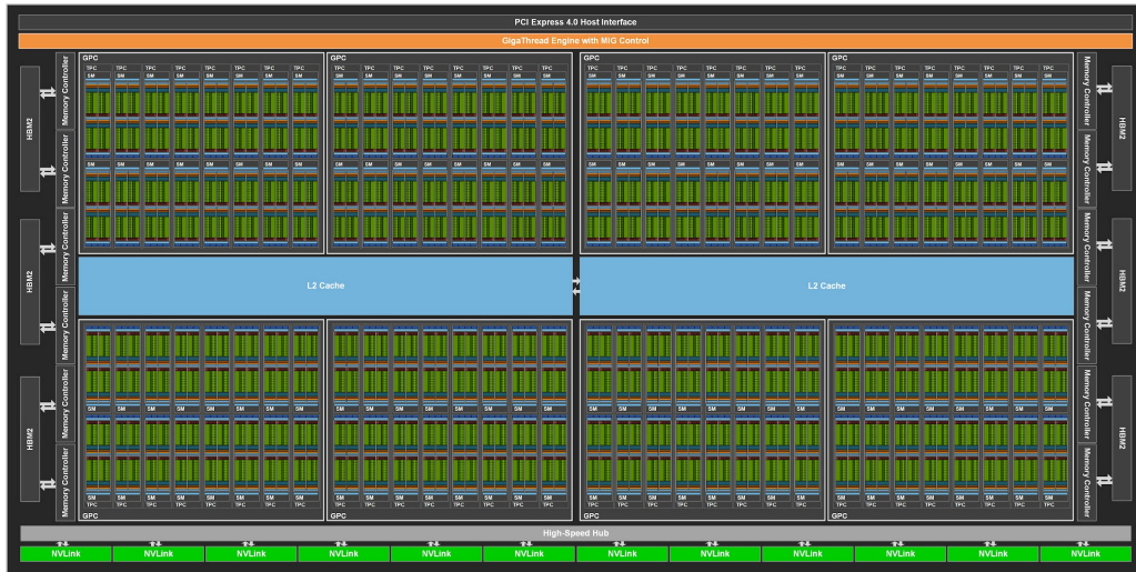
Figure 2.6: NVIDIA A100 GPU architecture
