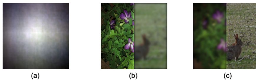
Fig. 4.4 Simulation of the (a) captured image; Reconstruction images (b) and (c) at different focusing distances.
