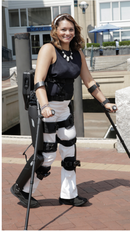
Figure 1.5: A person wearing the ReWalk Personal exoskeleton [23].
