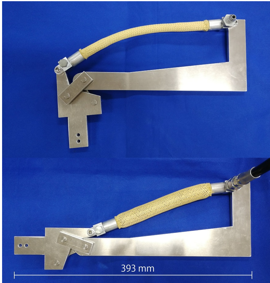
Figure 2.26: Photograph of the experimental device in unpressurized state and with 3 MPa applied pressure [99].
