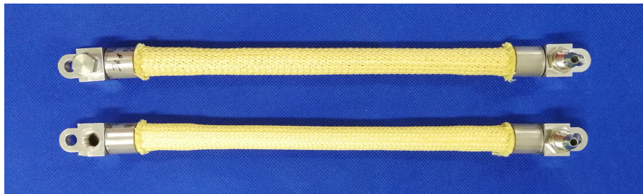
Figure 2.7: Photograph of both HAMs. The 25° HAM is shown on top, and the 30° HAM is shown on the bottom.
