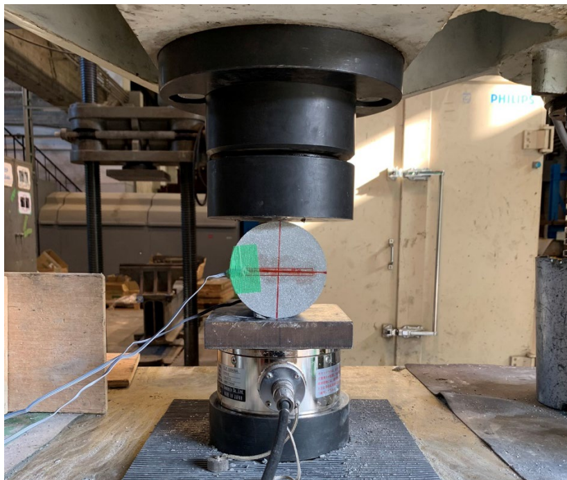
Figure 51 Split-tensile test experimental setup.
