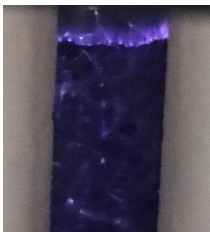
Figure 3.9 DBD generated in vertical PB-DBD reactor (i.d.=30 mm) at 40 kPa with Ru/Al 2 O 3 inside.
