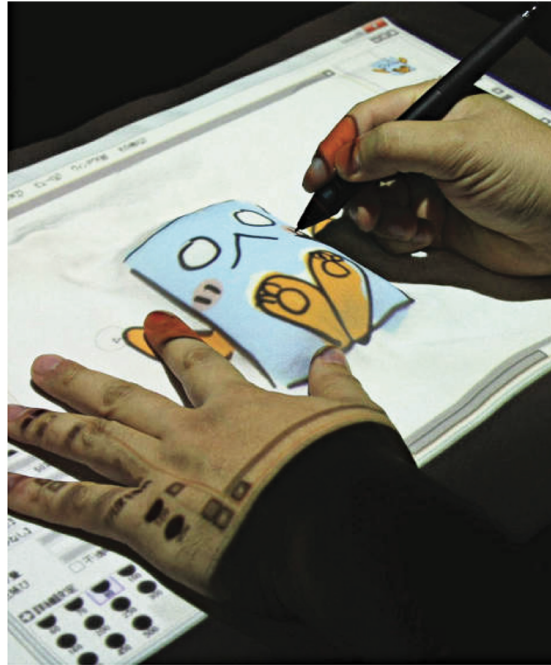
Figure 4.8: A person using the paint application. On the basis of the tactile feedback, users can employ the stylus to simulate different brush types
