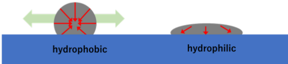
Figure. 5.5 Schematic illustration of drop size on hydrophobic and hydrophilic surface of Ph-BTBT-10 semiconductor layer and SiO 2 /Si substrate, respectively.
