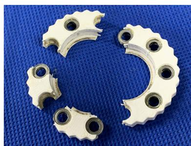
Fig.5 Broken planetary gear
