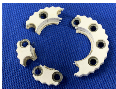
Fig.5 Broken planetary gear
