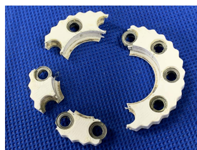
Fig.5 Broken planetary gear
