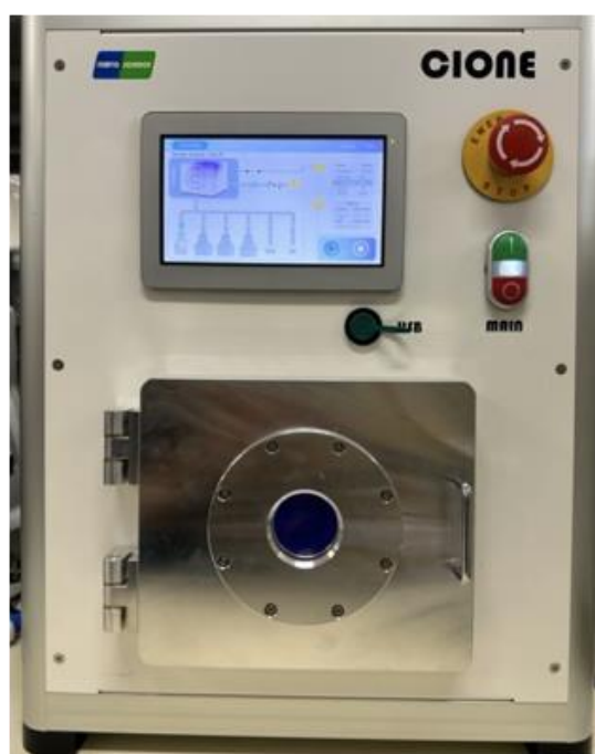
Fig. 2.2 Photograph of the plasma treatment device
