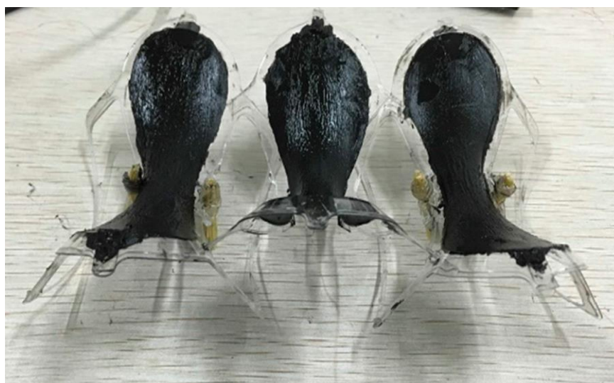
Fig.1.7 Annelid-robot made from a dielectric elastomer [6]
