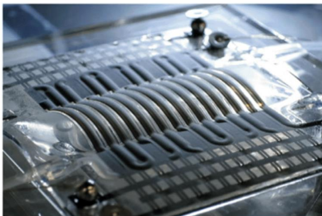
Fig. 1.5 Micro-conveyor with 28 integrated actuators [63]
