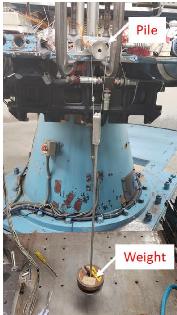
Figure 3.20: Simple model pile calibration test.
