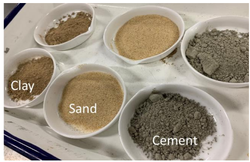
Figure 3.14: Material used for the modelling of the artificial soft rock.
