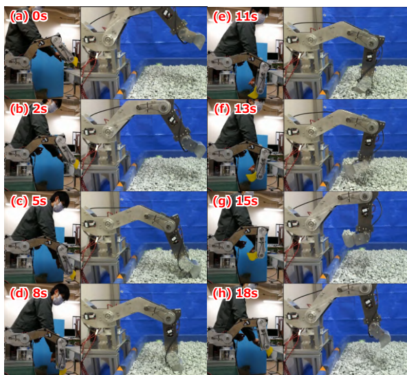
Fig.2.15 Experiment 3: Digging crushed stone
