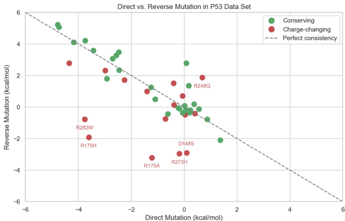
Figure 4.7: Internal consistency of direct and reverse mutations of the p53 data set. The green and red colors represent conserving and charge-changing mutations, respectively. The annotated points are the mutation cases where high inconsistencies are found.
