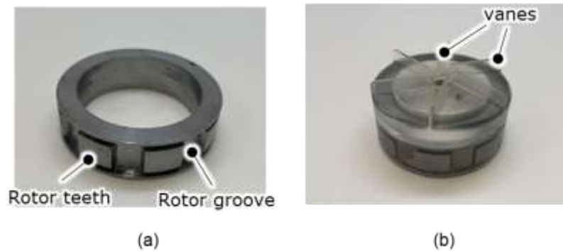
Figure 3.5 (a) Photograph of the iron rotor; (b) Photograph of the integrated waterproof impeller/rotor.
