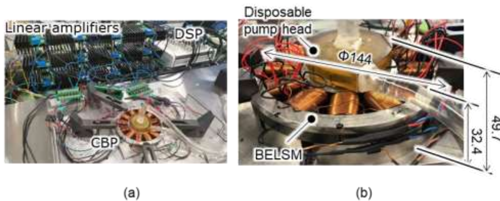
Figure 3.1 Photograph of the CBP system: (a) Entire system; (b) CBP utilizing the proposed BELSM.
