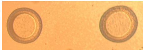
Fig. 3.2.14 n-contact etching and side-etching effects
