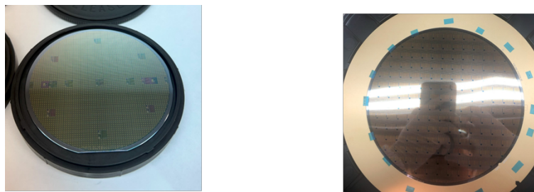
Fig. 3.3.1 Photo of VCSEL arrays made by 3-inch and 6-inch wafer-scale fabrication process
