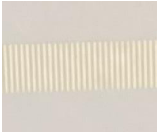
Fig. 6-4. The photo of surface grating
