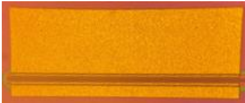
Fig. 6-12. The photo of the 2 nd order grating VCSEL
