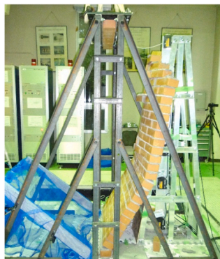
Fig. 15. OOP collapse of specimen CS.
