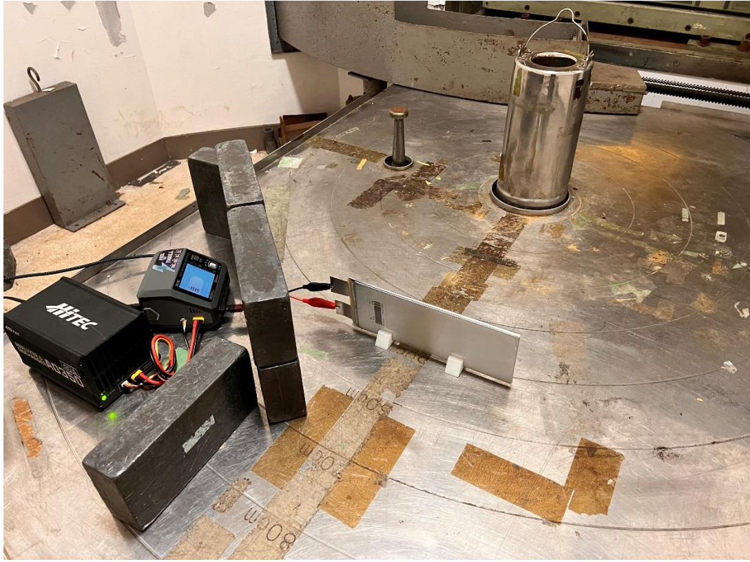
Fig.4.3 Photo of battery in irradiation chamber
