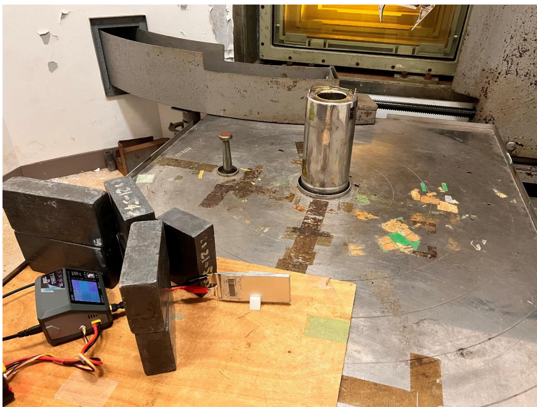
Fig.4.2 Photo of battery in irradiation chamber
