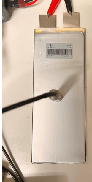
Fig 3.6 Measurement of All-Solid-State AMP-Battery Using Ultrasonic Transducer
