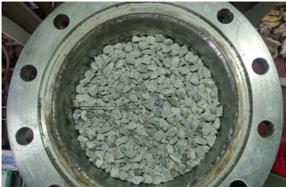
Fig.2.7 Photograph of the packed bed of rocks inside the storage tank
