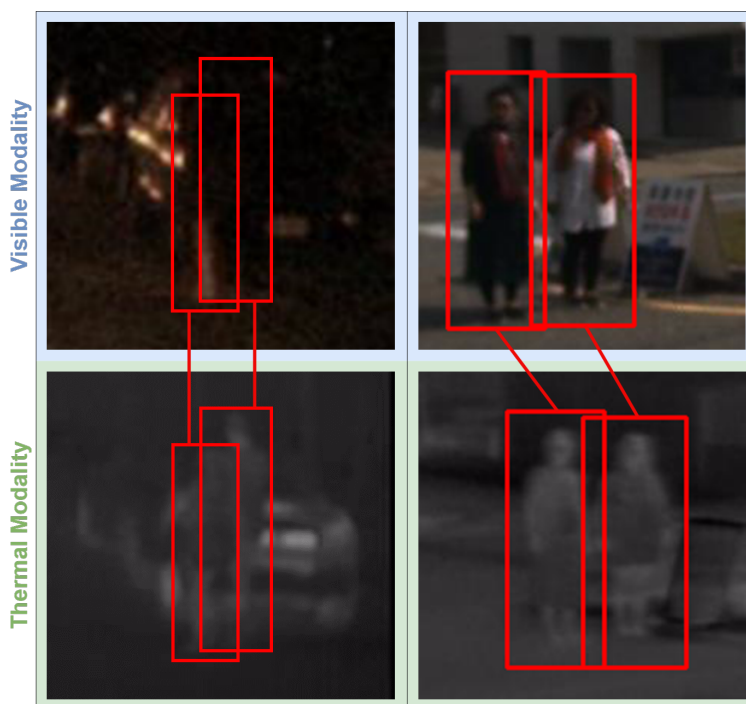
Figure 1.2: Examples of multi-modal pedestrian detection results. The left image pair demonstrates low brightness in the visible modality, making pedestrian recognition challenging, while the paired thermal modality facilitates detection. The right image pair illustrates misalignment, where the same pedestrians appear in different positions across modalities. Red boxes represent predicted bounding boxes, and lines between them indicate their paired relations.
